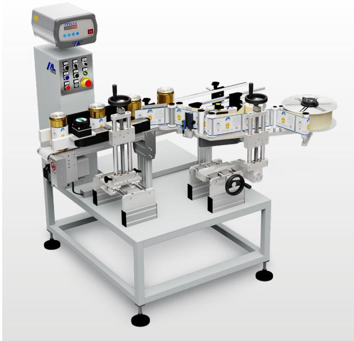
ALbelt C incorporates a specific set of additional devices which make ALbelt suitable for wrap-around labelling of cylindrical products.
